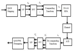
Fig.2.2 Block diagram of Companding techniques
