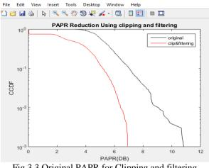
Fig.3.3 Original PAPR for Clipping and filtering
