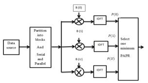
Fig.2.1The illustration block diagram of selective mapping Statistically independent is consider for each mapping, the CCDF of PAPR will be
