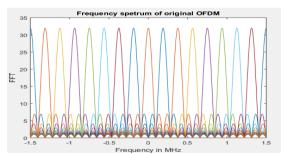
Fig. 1.1 Frequency spectrum of baseband OFDM system
